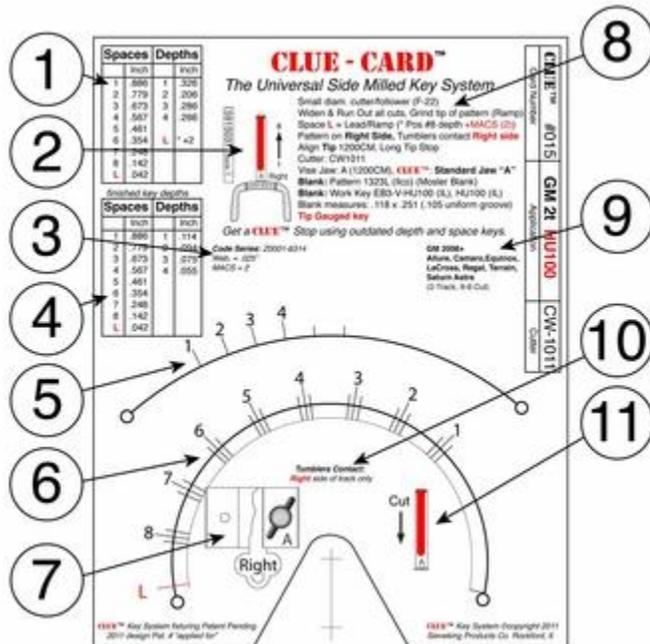
The Clue-Card™ has all of the information necessary to create the Pattern Key and cut the finished side-milled key.
