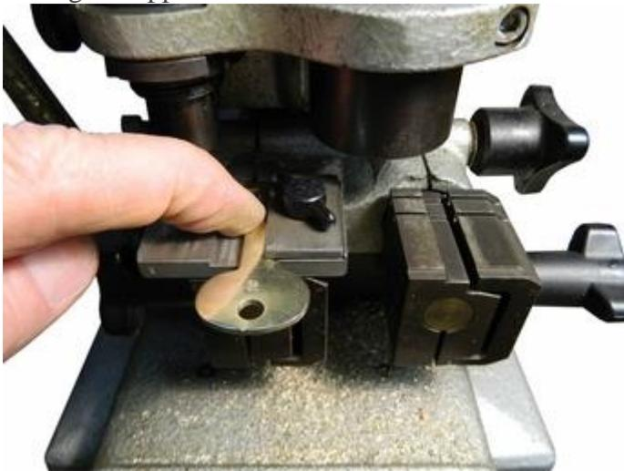
The **Clue™ Fixture and Pattern Key are Clamped** in the Pattern side Key Vise. The fixture is gauged using the Tip Gauge slot in the key vise. The key to be cut will be gauged using the same tip gauge slot.
