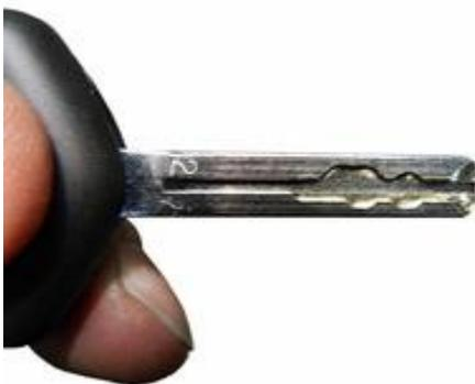
**The Finished Key.** Here is a perfectly cut Lexus four-track inside milled key. The depths and spacing are as accurate as the pattern that was used to create it. (Calibrate your 1200CM, to insure accuracy)
