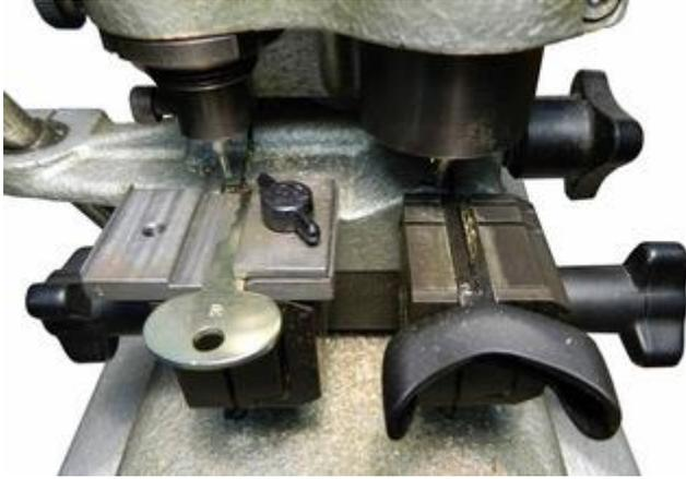
**Cut the First Track.** The First Track of the four-Track Lexus key being cut is made on the Right Track. This track is cut from Tip to Bow, for proper cutting direction. The key will be de-burred and reversed, to cut the Right track on the opposite side of the blank.
