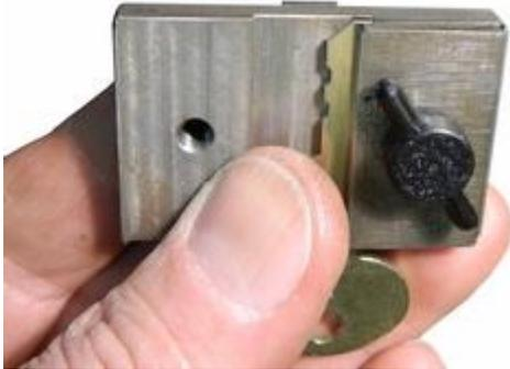
**Tip Gauge and Clamp the Pattern Key** in the Clue™ Fixture.
