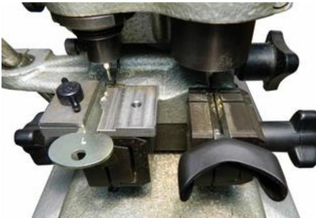
**Cut the Second Track.** The fixture has been reversed, to place the pattern for the Left Track at the Left side of the **Clue™** fixture. This track is cut from Bow to Tip, for proper cutting direction. This key will be de-burred and reversed, to cut the Left track on the opposite side of the blank and complete the key cutting process.
